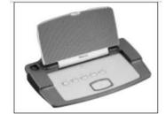
The LBB 3544/00 is the standard delegate conference unit, enabling delegates to speak, register a request-to-speak, register a response request, listen to the speaker and vote. The flat-panel loudspeaker offers superior acoustics with minimal feedback, so increasing intelligibility. It is automatically muted when the microphone is activated. When the
